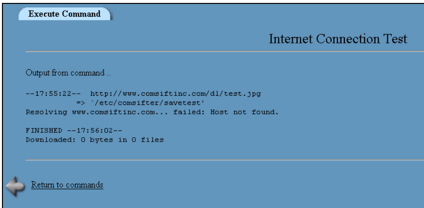
Figure 3-23: Failed DNS Screen
